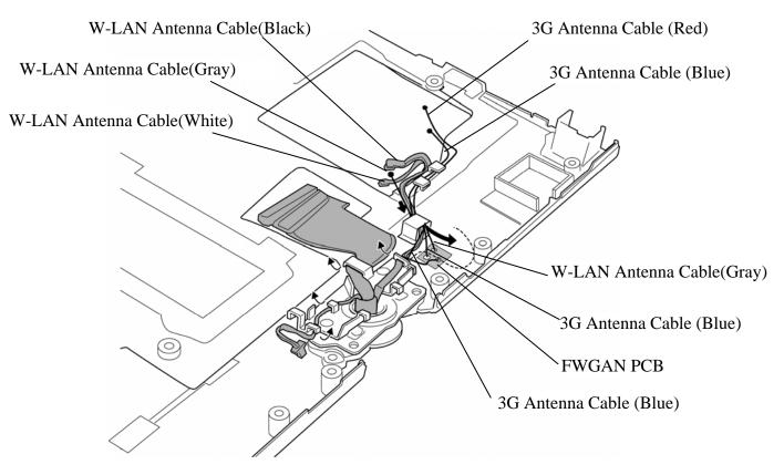
Figure 4-49 Removing the hinge assembly (1) (3G model only)
